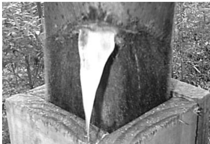
Image 15: Producing square section bamboo culms
