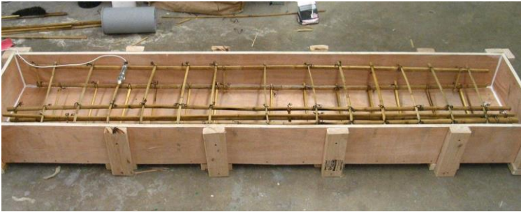
Image 14: Bamboo reinforced concrete beam
