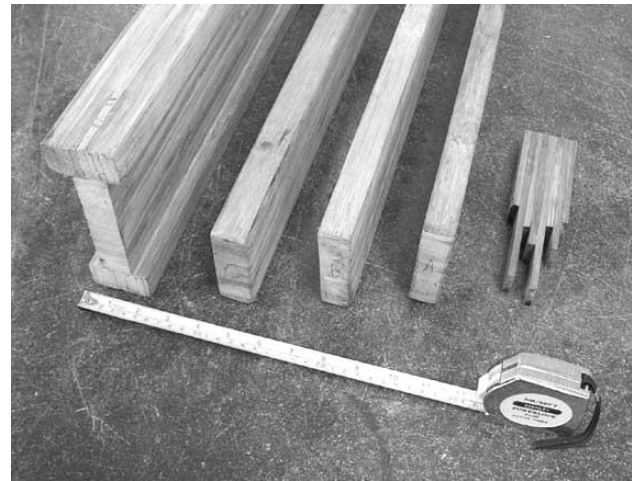
image 20: Various sections of laminated bamboo beams
