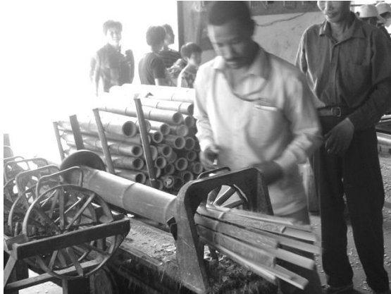
Image 12: Mechanical splitting of a bamboo culm
