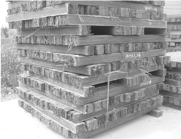
Image 21: Reconstructed bamboo timber
