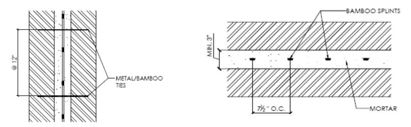
Image 15: Bamboo reinforcement for cavity wall construction
