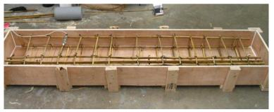
Image 14: Bamboo reinforced concrete beam
