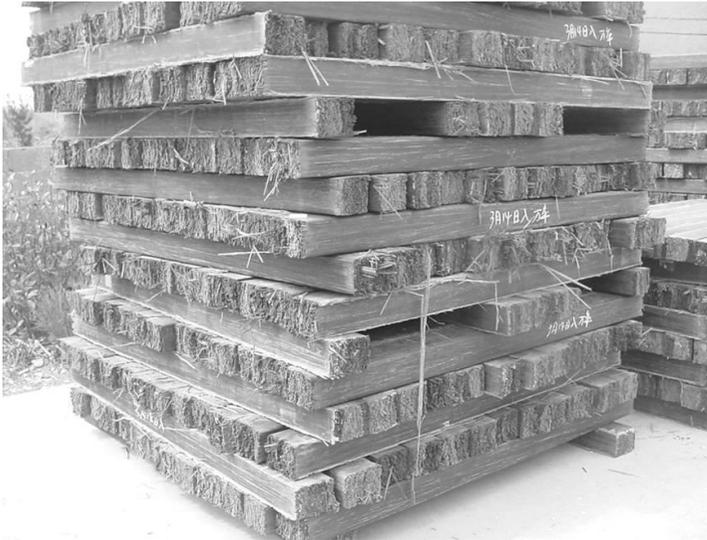
*Image 21: Reconstructed bamboo timber*
