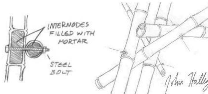
Image 27 :Connections with thread rods and mortar injections
