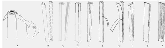
Image 10: The process of splitting the bamboo manually
