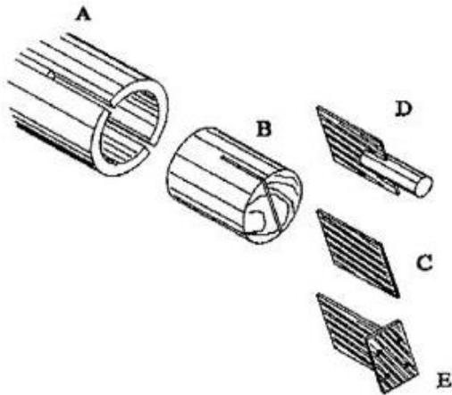
*Image 26: Wood core insertion and steel plates*
