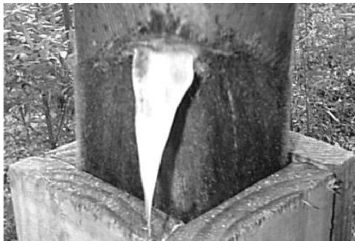
Image 15: Producing square section bamboo culms
