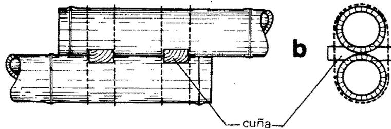
*Image 24 : Connecting two horizontal elements*
